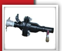
The Mix Mateprovides rapid and thorough mixing of two or more liquid streams. Especially effective as a sludge-polymer mixing device, the Mix Mate® produces uniformly flocculated sludge ready to be dewatered. Standard units handle flow rates in the 10 - 400 GPM range. The units are constructed of carbon steel body with a rubber nozzle plate. Other materials of construction are available upon request.
